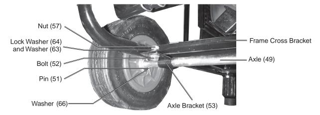
7. Place each Wheel (50) over the end of the Axle and secure in place with another Pin (51). Bend Pin so it cannot fall out.
